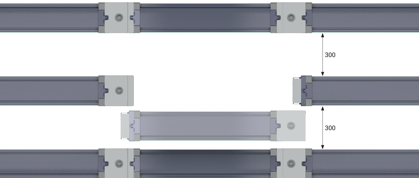
FIGURE-4 MINIMUM DISTANCE BETWEEN BUSBAR RUNS
